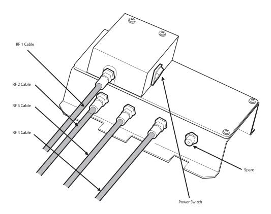
Figure 12. Cable Connection on Power Switch Box
