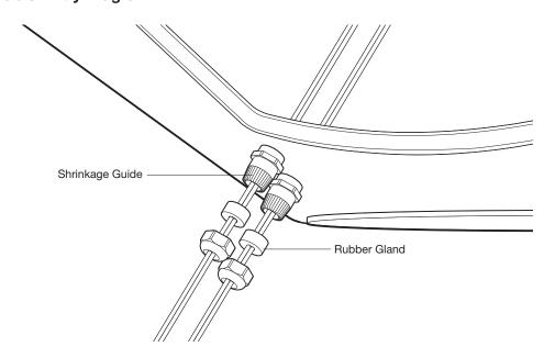
Cable Entry Diagram through Side Holes
