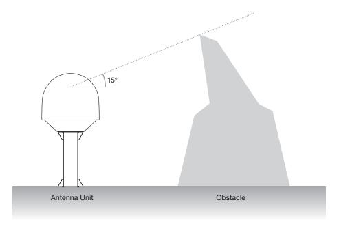
Figure 05. Elevation Limit of Obstacle
