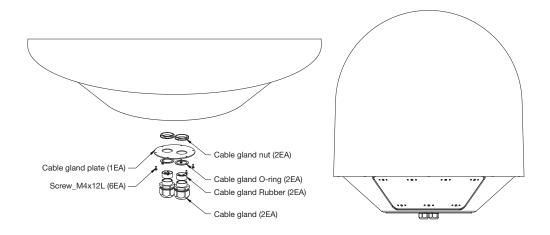
Figure 07. Cable Gland Assembly
