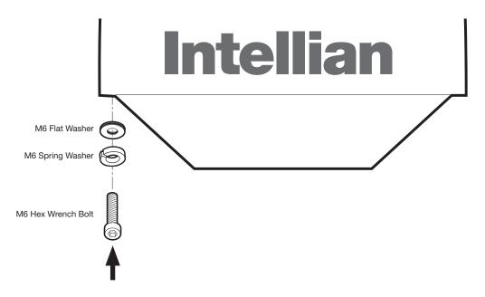
Figure 13. Top Radome Reinstallation
