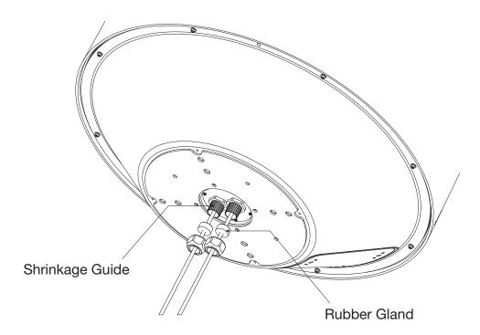
Figure 08. Cable Entry Diagram
