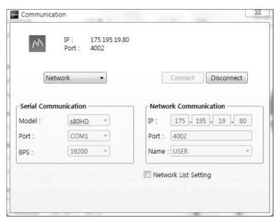
12. Click on Comm. icon to open the communication window. Assign the correct COM Port (step 10) and click the "Connect" button.
