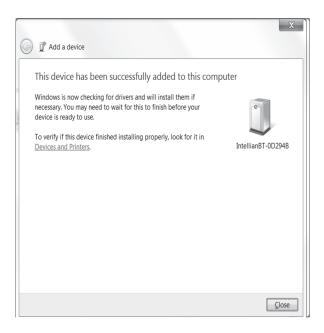
7. Pairing completed, the bluetooth device has been added to the computer. With Generic Serial Setup for OS systems that are different from Windows 7, go to a Generic Serial Service page (which applies to some OS Systems), select the Generic Serial Service and click Next.
