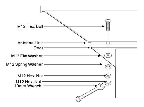
Figure 11. Mounting Components Diagram
