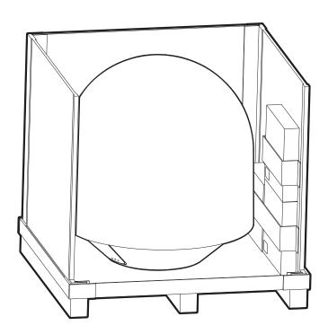
**Step 3.** Remove the 4 shipping bolts that mount the antenna to the pallet.
