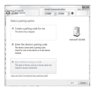
5. Pair the device without using a code. Select "Pair without using a code" and press Next.
