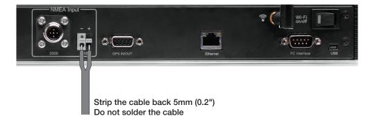
Figure 17. Gyrocompass Connection
