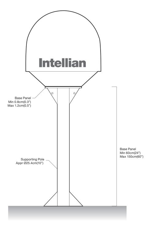
Figure 10. Recommended size of the support pedestal
