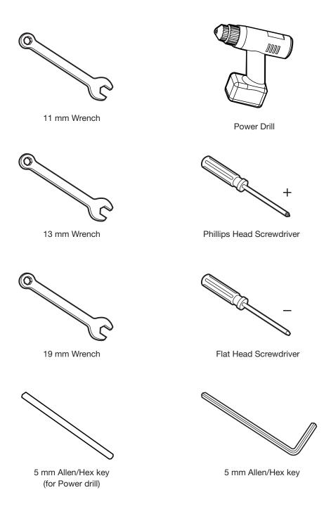
Figure 06. Tool Sets for Installation
