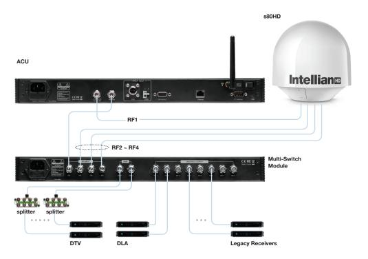
Figure 01. Basic System Configuration
