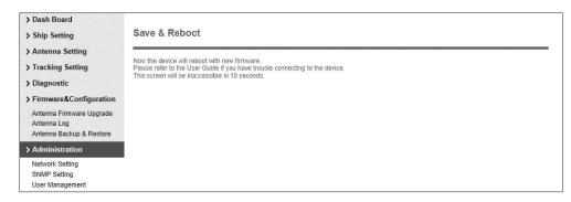
6. The connection will be disconnected during the reboot. It'll take around 30 seconds to reboot the iARM module and get the connection back again. (Disconnection message may vary depending on the web browsers.)
