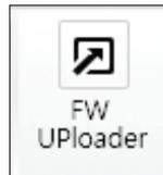
**FW Uploader:** launches firmware upload wizard to upgrade Antenna and ACU firmware from a PC. Connect the PC to the ACU via a USB cable and follow instructions on the Wizard until the firmware upgrade is complete.
