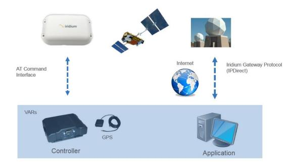
Figure 2-2 Iridium Edge Integration in an Application
