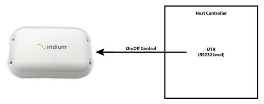
Prior to turning off the Iridium Edge, a "flush memory" (AT\*F) command should be issued to ensure all internal SBD modem's flash memory write activity is completed.
