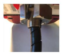
• Firmly press the sheath so that it makes contact with the Iridium Edge's baseplate and goes inside the Slotted Screw.
