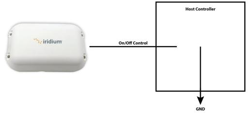
Alternatively, the On/Off control line can be driven directly by a RS232 signal level such as DTR.
