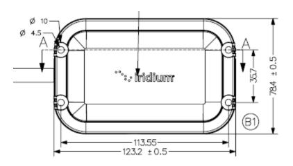
Figure 2-9 Enclosure Side View
