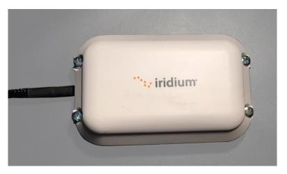
Secure all mounting nuts with an appropriate thread locker that meets the installation requirements for factors such as vibration and temperature
