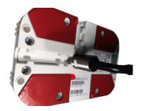
• Carefully press the Rubber Grommet into the baseplate until it is flush with the Iridium Edge.
